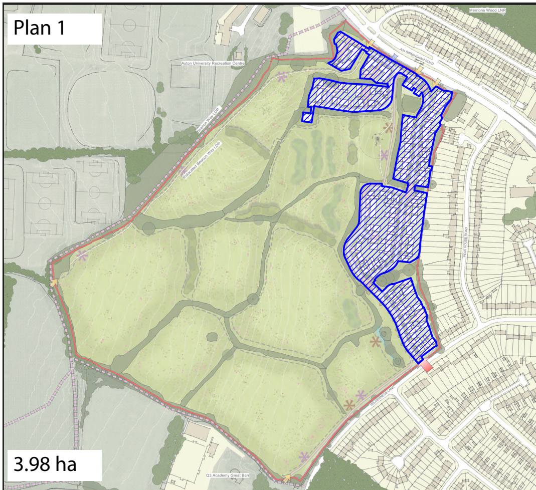
Developed areas and roads measured only. Retained vegetation, play area, SUDS excluded.
