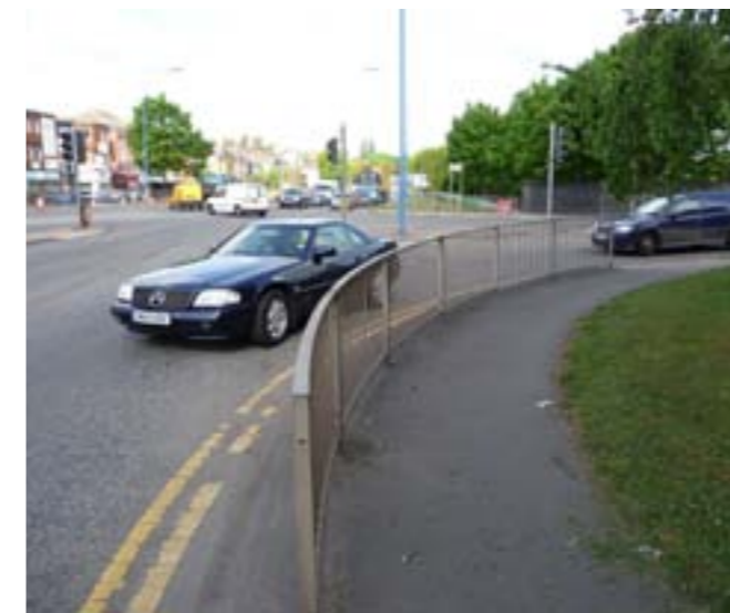
Large-radius slip road privileges vehicular movement
