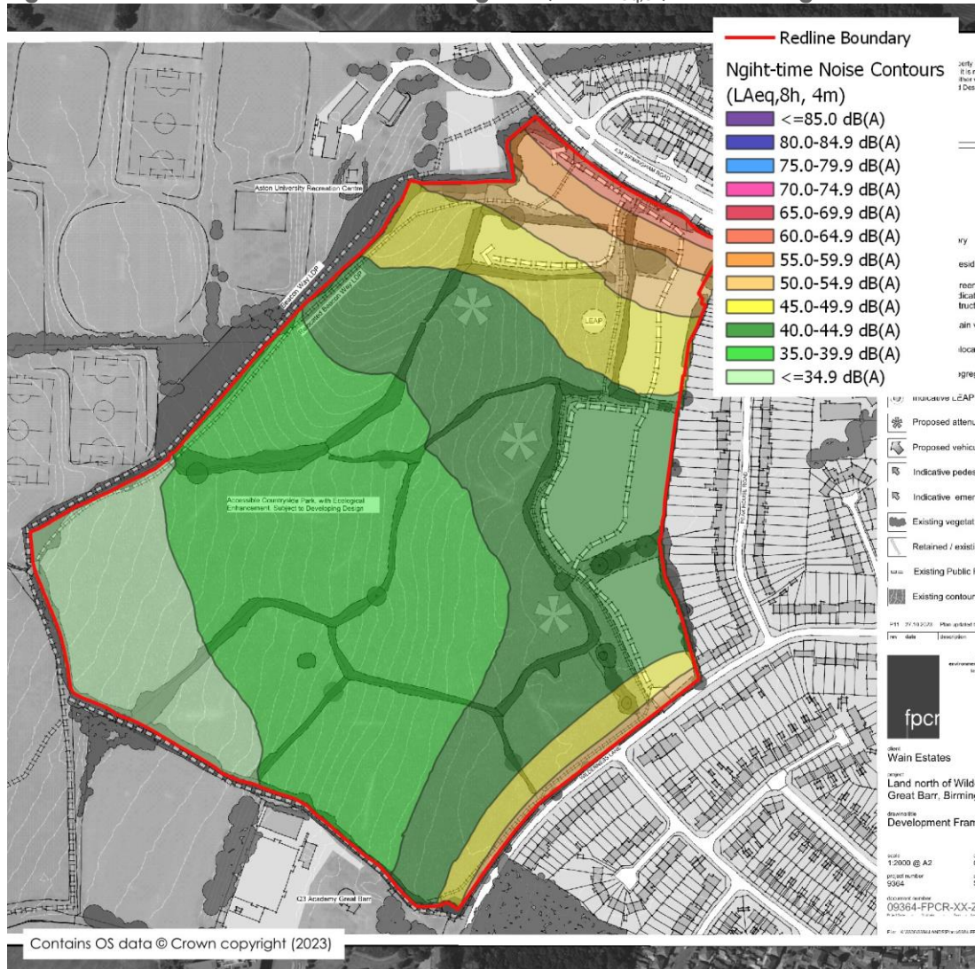
Figure 4.2: Noise Contour Plot without Mitigation, dB LAeq,8h, 4m above ground
