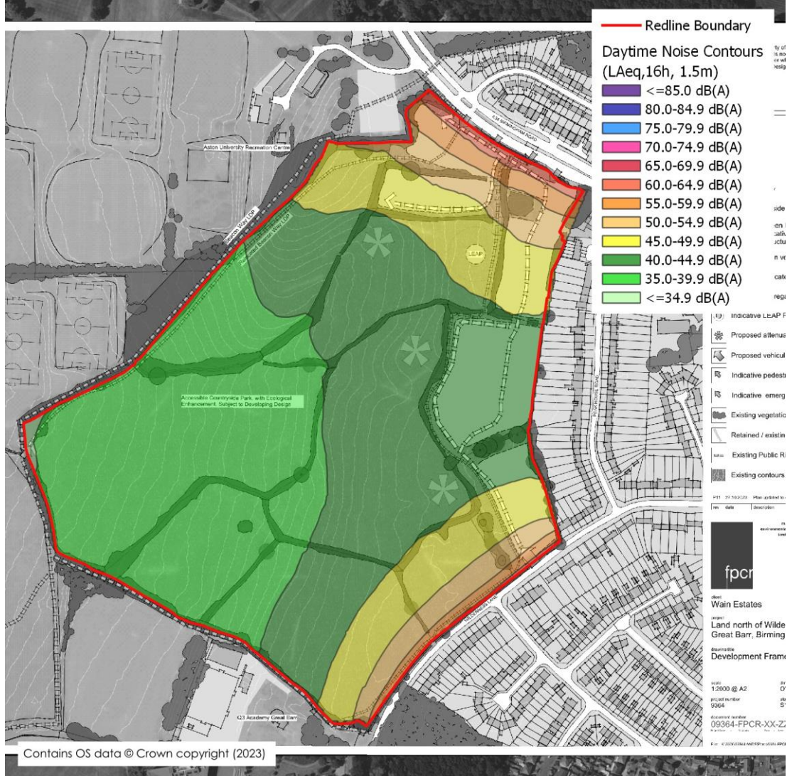
Figure 4.1: Noise Contour Plot without Mitigation, dB L_{Aeq,16h} , 1.5m above ground
