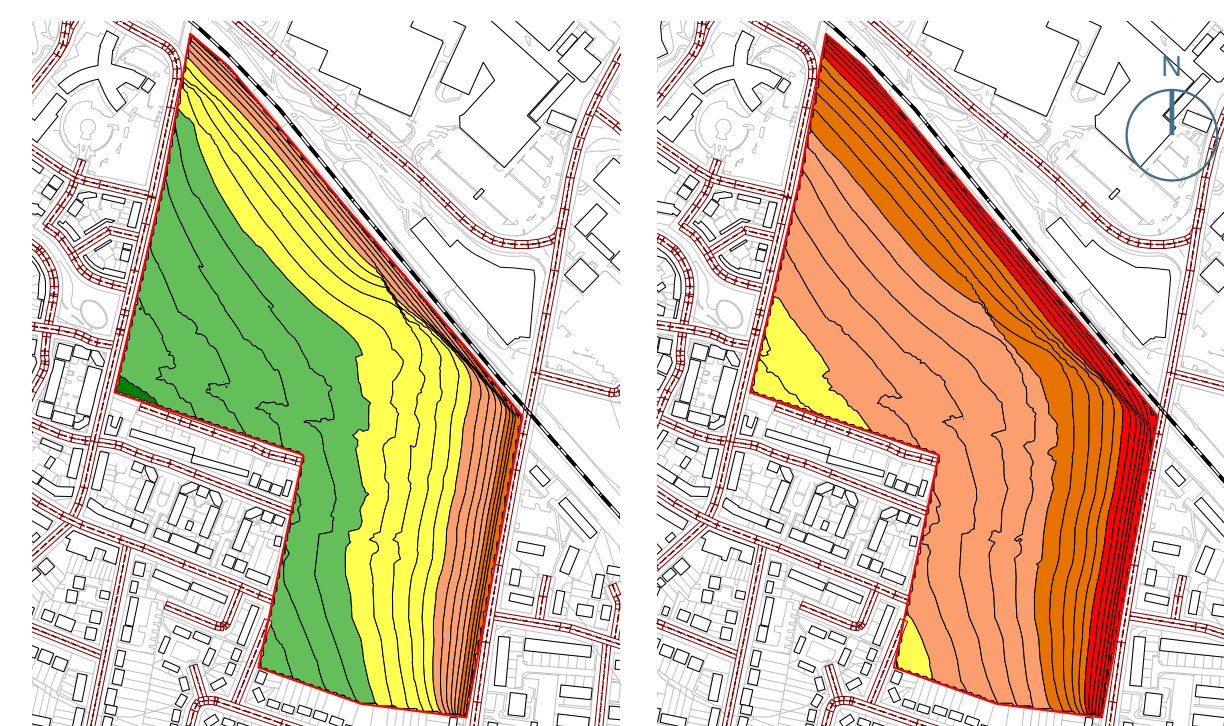
Extracts from noise assessment, showing noise pollution during the day (left) and night (right)
