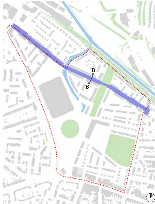
Fig. 5.25 - Cranford Street widened to accommodate the cycle route on its southern side, overlaid on masterplan
