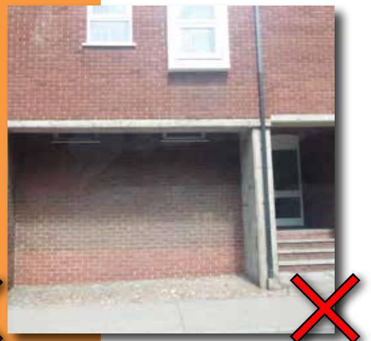
Bad response to the street frontage resulting in a poor quality space, lack of natural surveillance and legibility.
