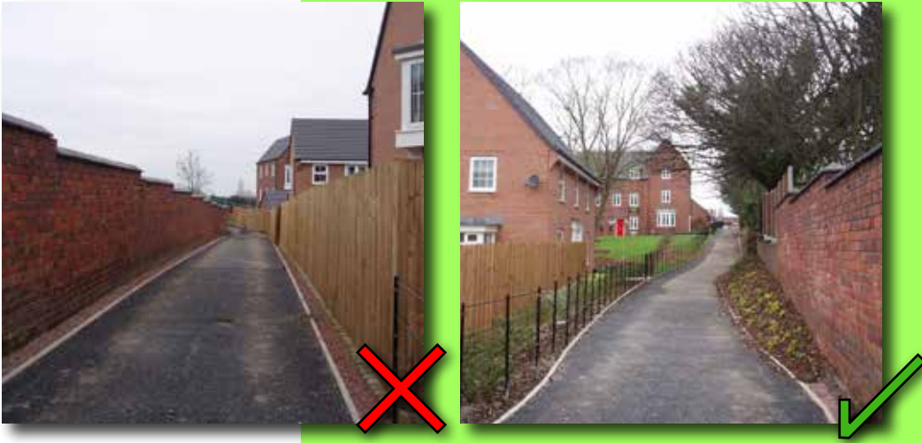
Avoid segregating pedestrian routes where they are not overlooked by active frontages and which therefore feel unsafe.
