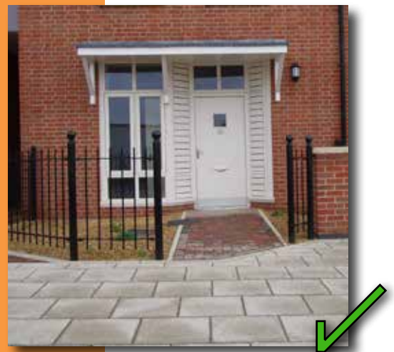
Good Example of frontage design, deep lounge window fenestration overlooks the street and the the garden has a clear boundary. Note also the removal of the service box of the facade of the dwelling which is hidden behind the boundary wall.
