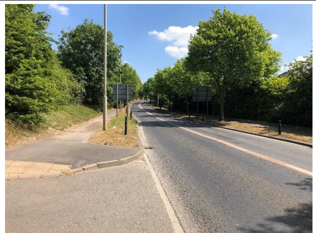
Photo 2 – Potential verges to accommodate cycling infrastructure on Stallings Lane, but constrained by trees in the verge
