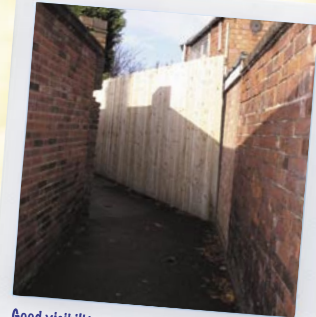
Good visibility at both ends of passageways is required. 'Doglegs' should be avoided.
