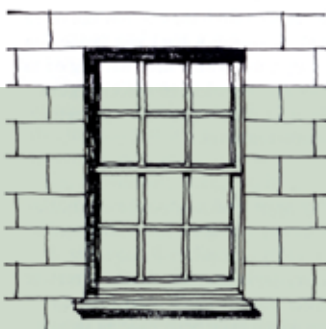
Typical late eighteenth century window. Frame set back from wall face and recessed behind reveals. Very slender glazing bars.
